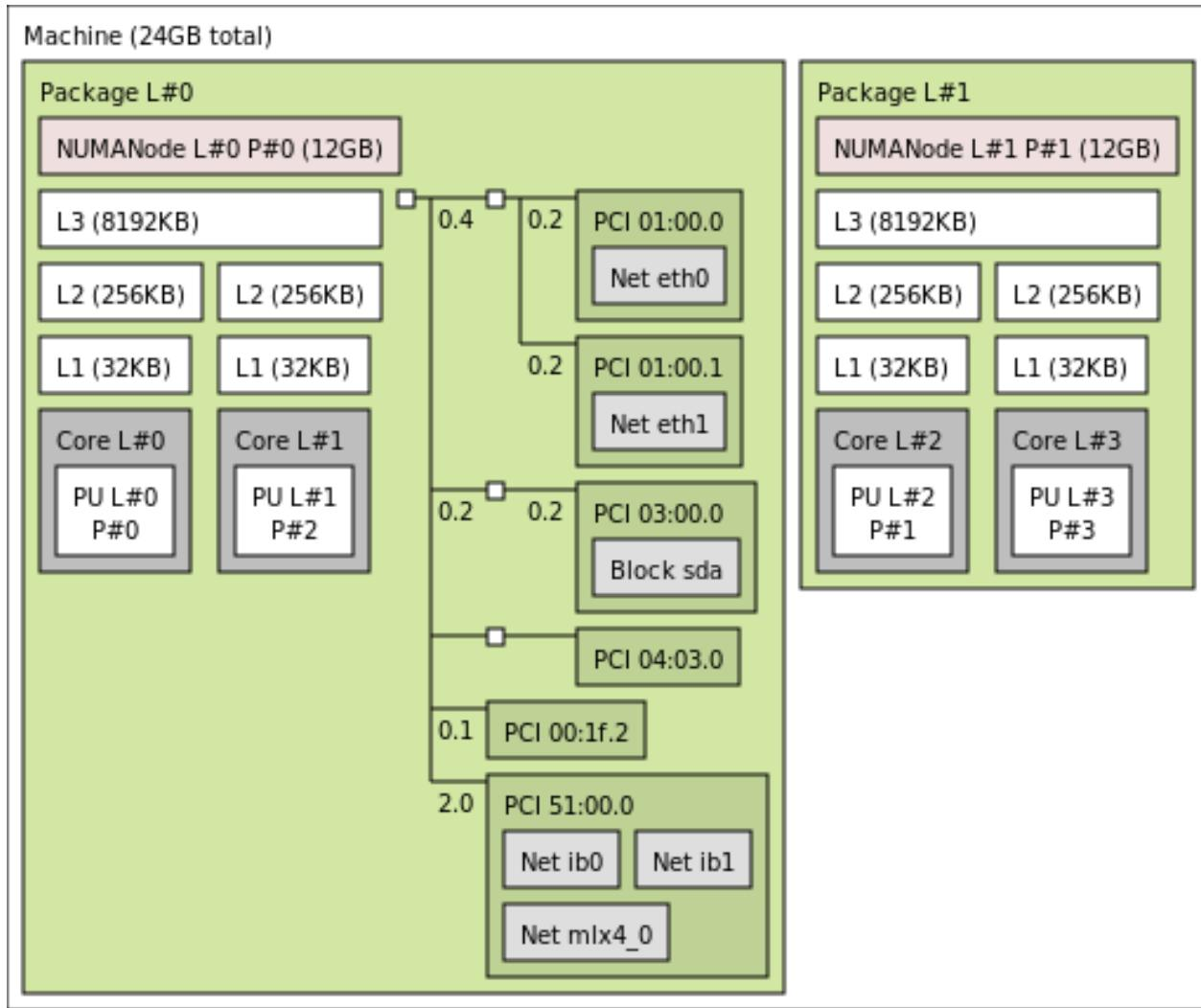
Six interesting PCI devices were discovered (dark green boxes). However, hwloc found some corresponding software devices (*eth0*, *eth1*, *sda*, *mlx4\_0*, *ib0*, and *ib1* light grey boxes) for only four of these physical devices. The other ones (*PCI 04:03.0* and *PCI 00:1f.2*) are an unused IDE controller (no disk attached) and a graphic card (no corresponding software device reported to the user by the operating system).
